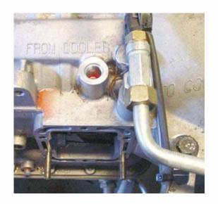
\*After fastening the high pressure line to the transmission, circuit need to be checked
